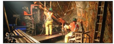
Drilling for Molybdenum from an underground tunnel
