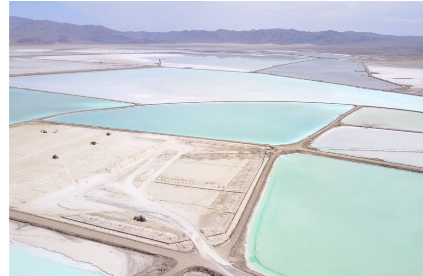
The oldest active lithium production site in the USA is Albemarle's Silver Peak solar evaporation mine, which has been active since the 1960s. CLUI photo
