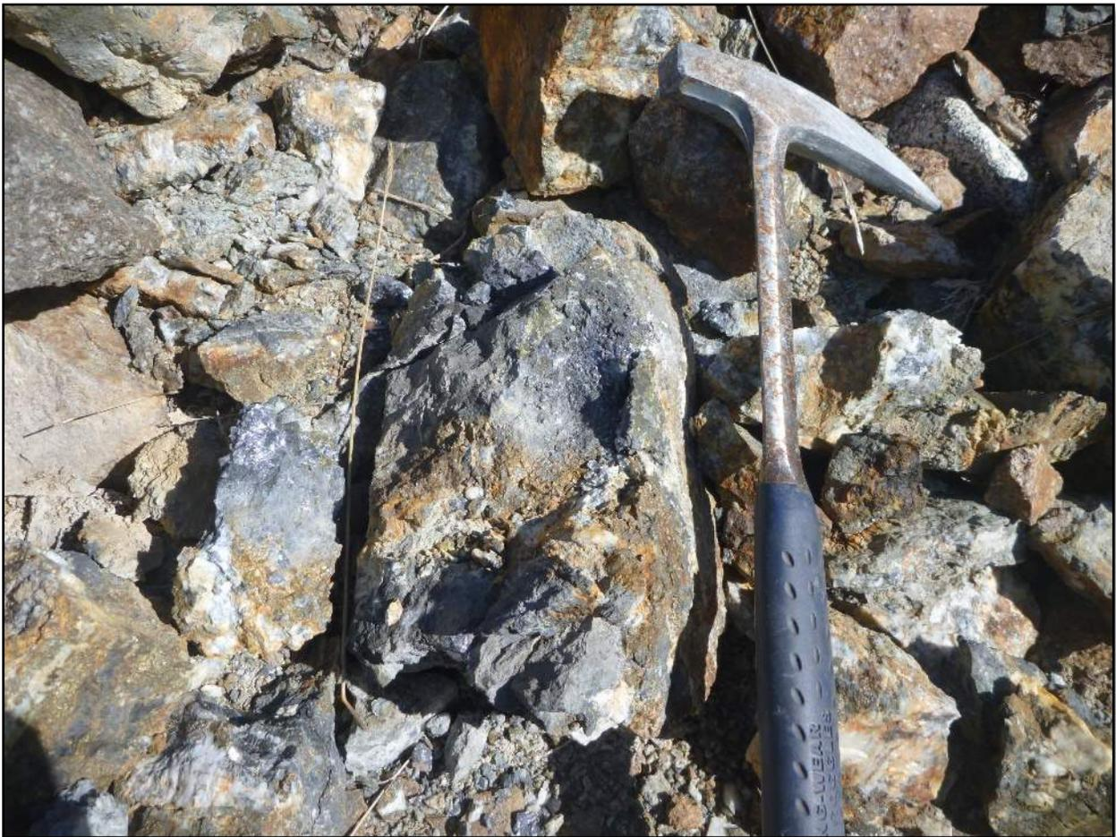
**Figure 4: Massive galena and sphalerite, 47-Zone**
